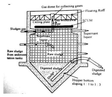
It cold courtiers the tank may have to be provided with heating coils through which hot water is circulated in order that the temperature inside the tank is maintained at optimum digestion temperature level.
